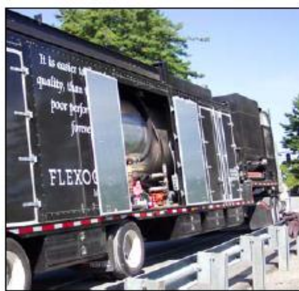
Side view of Polycarb's truck (note resin and catalyst storage tank).
