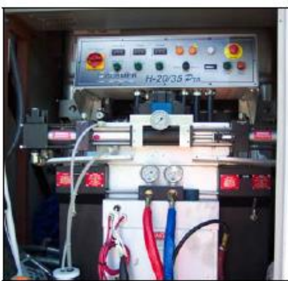
Onboard computerized blending system on Polycarb's truck.
