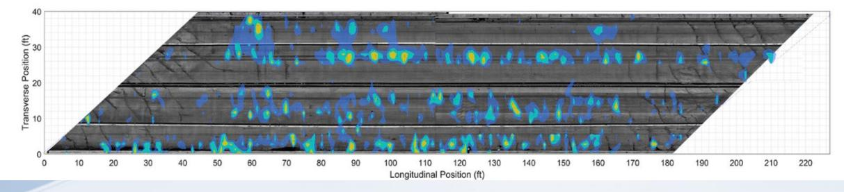
Areas with sealed cracks show lower changes in dielectric constant compared to the background.
