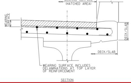
**Defect 3210** IR/Thermography or GPR Results for delaminations down to the top layer of reinforcement should be quantified under Defect 3210 under the applicable wearing surface element.
