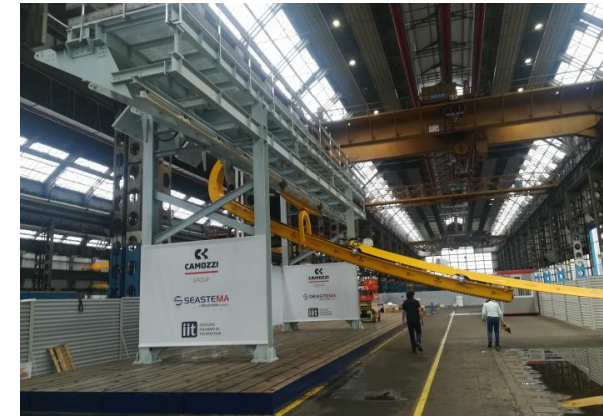
TESTS CONDUCTED IN THE CAMOZZI FACTORY IN MILAN ON A 1:1 SCALE BRIDGE MOCKUP
